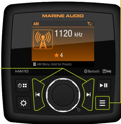
**RADIO MENU:** Press to enter radio menu. Rotate the VOL/ENTER knob to navigate through radio menu items: PRESETS, SCAN PRESETS and AUTOSAVE PRESETS.
